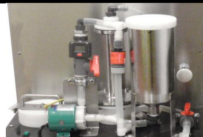
2 PEF cell, 1.5l batch, reg. pump, flow meter:
