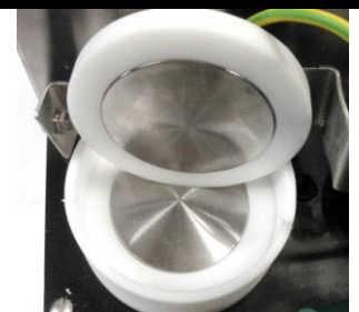
PEF cell with parallel electrodes:
