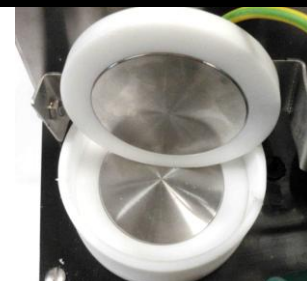
PEF cell with parallel electrodes:
