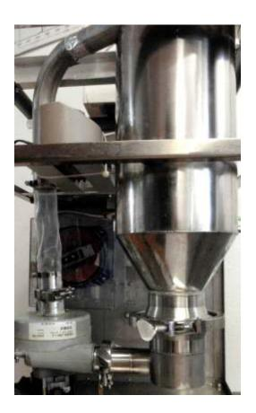
The system was tested on various spice and powders. It has shown 1 to 3 logs reduction (in Total Plate Count, TPC) in shred teas, spices and some powders at 100-450 wh/kg (5-20c/kg).
