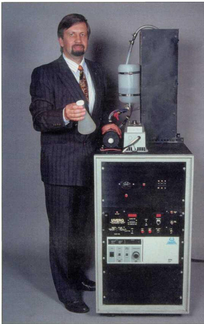
Physicist Alex Wekhof's UV destruction process relies on a phenomenon known as direct photolysis, where UV light dissociates, or decomposes, organics.
