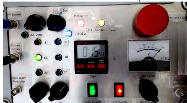
One of custom PEF control panels
